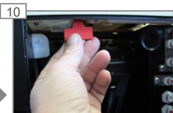
Push the locking slide all the way in.
