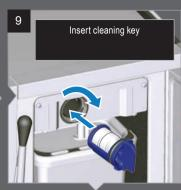
Cleaning procedure starts automatically after the cleaning key is inserted.
