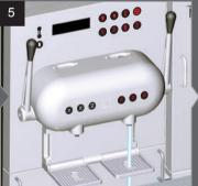
Automatic internal rinsing: An approx. 3 sec. internal rinsing of the milk system will begin immediately after each milk-based beverage preparation.
