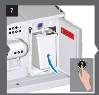
Place empty container back into the refrigerator and guide the suction tube with temperature sensor and level sensor into the container. Press any button.
