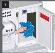
Carefully wipe milk suction tube with temperature sensor and level sensor, using only singleuse disposable tissue or paper towel.
