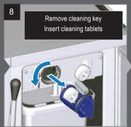
Remove cleaning key and insert two cleaning tablets.
