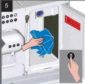
Carefully wipe milk suction tube with temperature sensor and level sensor, using only single-use disposable tissue or paper towel. Afterwards press any button.
