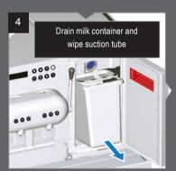
Carefully remove and drain the milk container.
