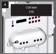
Machine performs a cold start rinse (display shows a counter of 3 min.).
