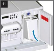
Insert milk suction tube with temperature sensor and level sensor through cover into the milk container.
