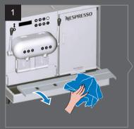
Remove the drip grid and wash it with a soft cloth and mild detergent under running
