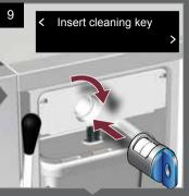
When key inserted cleaning starts automatically.
