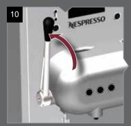
By pulling up the lever, the used capsule is ejected.
