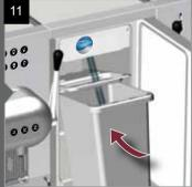
Insert milk suction tube through cover into the milk
