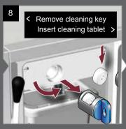
Remove cleaning key and insert two cleaning tablets.
